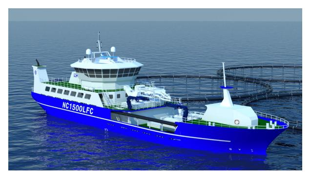
LOA - 60,5m LPP - 55,5m B -14m D MAIN DECK -6,0m D BOAT DECK -8,8m T MAX - ~5,3m Frame spacing - 0,6m
